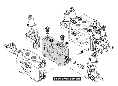
EX38 has been conceived as a post compensated flow sharing valve, but completely interchangeable pre compensated sections are also available.
