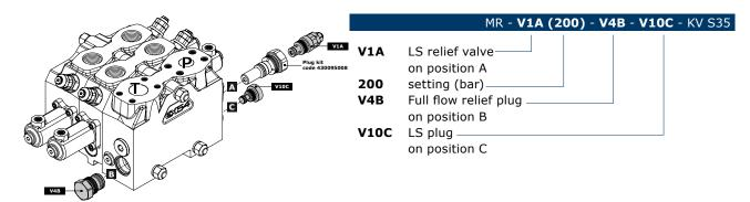
**NOTE**: quires minimum 40 bar difference in setting of valve V1A (LS relief valve) and alve V3B (Full flow relief valve)
