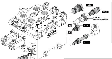
In the presence of LS pressure relief valve (V1A) is compulsory to order separately plug adapter kit that allows the correct assembly of the valve on the inlet section.
