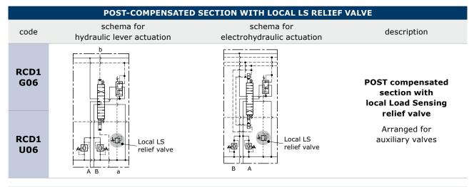
NOTE: RCD1 type in combination with HP04, HP07, HP08, HP09, HP01 requires left inlet assembly (ML).
