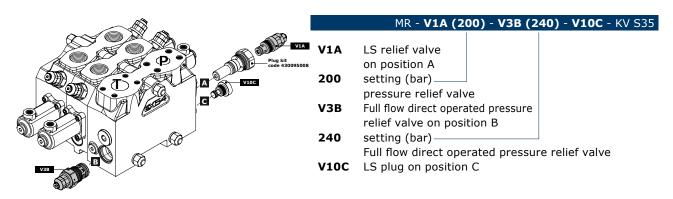
**NOTE**: when ordering a valve type V11C, it is necessary to specify connector type (see table "A" page 18)
