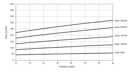
$\label{eq:post-compensated} Post compensated spool flow characteristic Fixed displacement systems (KV): flow on ports A and B as function of spool stroke, pilot pressure, control current Inlet flow: 300 l/min - Pump inlet compensator at 16 bar <math display="inline">\Delta p$
