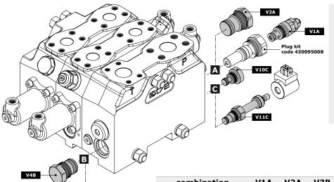
In the presence of LS pressure relief valve (V1A) is compulsory to order separately plug adapter kit that allows the correct assembly of the valve on the inlet section.
