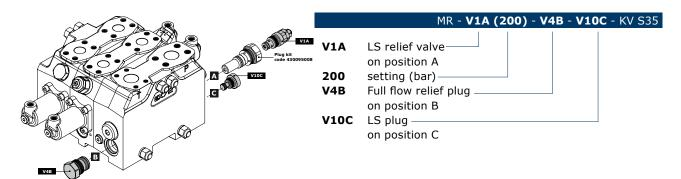
**NOTE**: quires minimum 40 bar difference in setting of valve V1A (LS relief valve) and alve V3B (Full flow relief valve)
