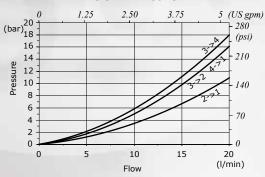
ET10L Pressure drop vs. flow (spool 1 type)
