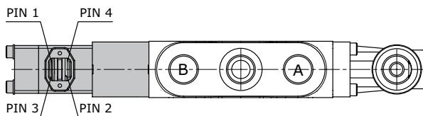
**CONTROL in A e B** = connect PIN 1 - 4 and 2 - 3
