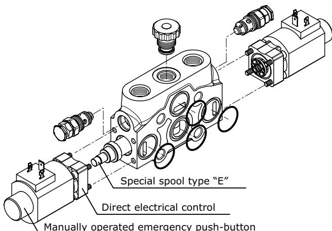
The H036 and H037 direct electric controls come as two kits each including a: coil, spring, solenoid and adapter.
