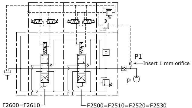
Proportional control kit, mechanically retrooperated, allows the maximum precision of positioning, limiting the hysteresis. The control is operated with PWM control of the current. PWM frequency suggest: 60-80 Hz
