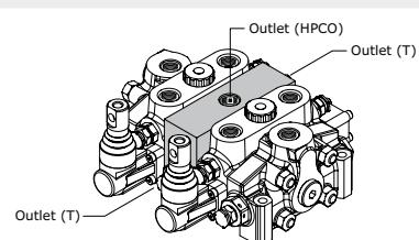
Upper outlet HPCO front side A and rear side B to T
