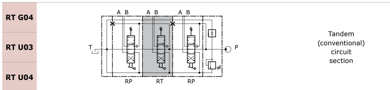
When the spool is operated it intercepts the switch gallery by diverting the flow of oil to service port A or B. The Tandem circuit is powered by the switch gallery thus permitting the use of just one work section at a time. The section downstream from the tandem section that has been actuated does not operate, the upstream section has priority.
