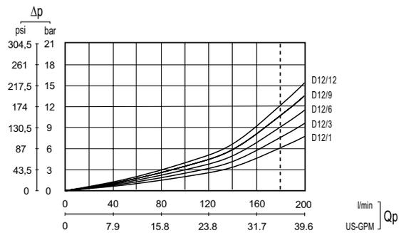
Pilot operated relief valve curve
