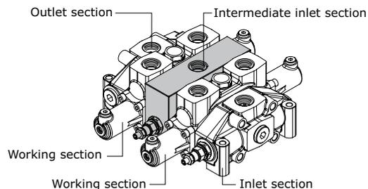
**Complete configuration samples for D12/2 with intermediate inlet section (BV)**
