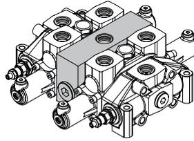
Intermediate outlet section with **single tank return**
