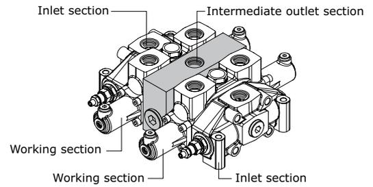
**Complete configuration samples for D12/2 with intermediate outlet section (BG)**
