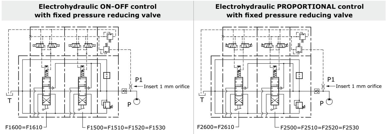
Proportional control kit, mechanically retrooperated, allows the maximum precision of positioning, limiting the hysteresis. The control is operated with PWM control of the current. PWM frequency suggest: 60-80 Hz
