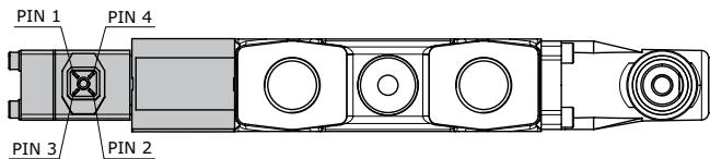
**CONTROL in A e B** = connect PIN 1 - 4 and 2 - 3
