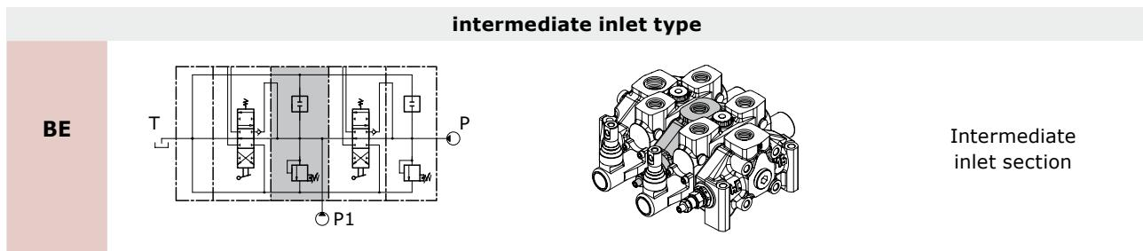
The intermediate inlet section is driven by two pumps (P + P1). The downstream elements can be set to a lower pressure than the upstream ones by adjusting the pressure relief valve of the intermediate section in question.
