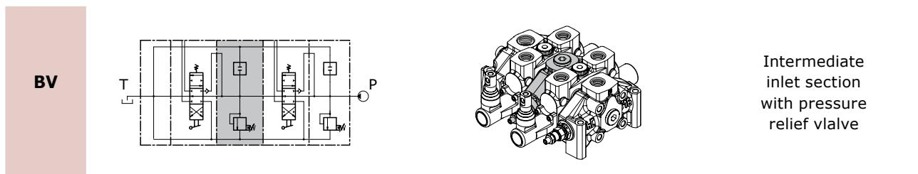
The intermediate inlet section and the elements are driven by a single pump (P). The downstream elements can be set to a lower pressure than the upstream ones by adjusting the pressure relief valve of the intermediate section in question.
