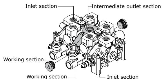
**Complete configuration samples for D16/2 with intermediate outlet section (BG)**
