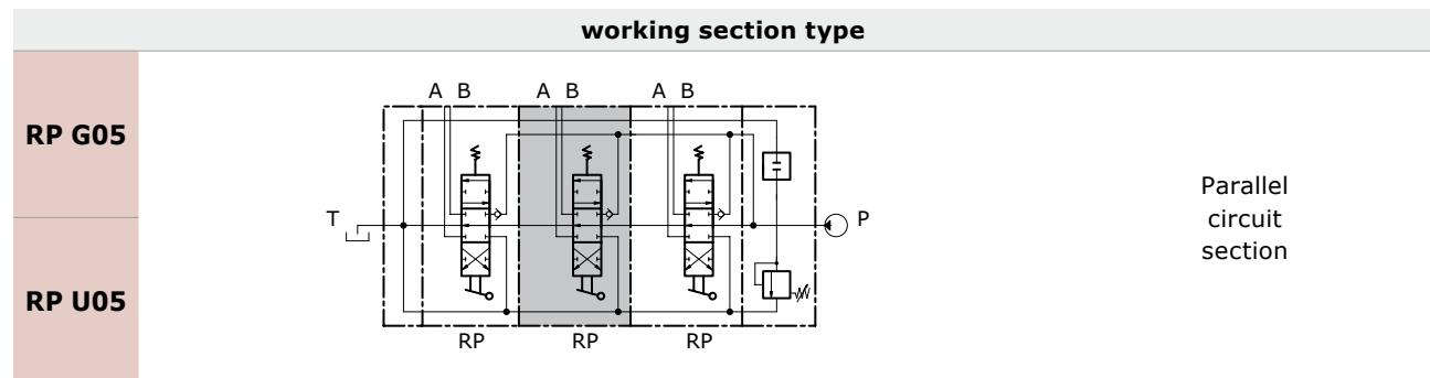
When the spool is operated it intercepts the by-pass gallery by diverting the flow of oil to service port A or B. If two or more spools are actuated at the same time, the oil will power the service port that has the lower load; by throttling the spools, the flow of oil can be divided between two or more service ports.
