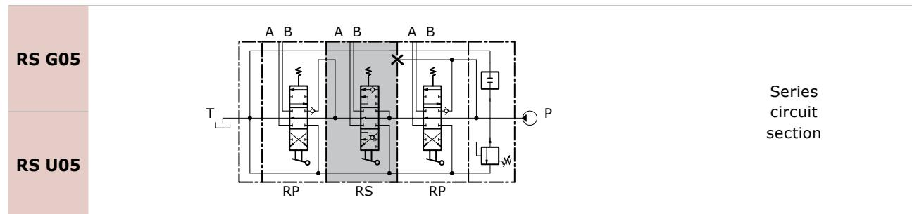
When the spool is operated it intercepts the switch gallery by diverting the flow of oil to service port A or B. The oil that flows back from the actuator is carried to the switch gallery thus making it available to the service ports downstream from the series section. The pressure drop downstream is added to the pressure drop of the section itself.
