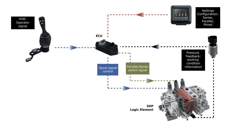
The work mode can be simply set by selecting it on the control panel.
