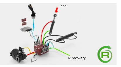
Recovery during simultaneous functions
