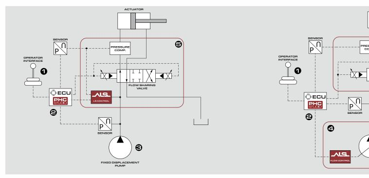
This solution enables to use Pressure Control functions paired with Flow Sharing directional control valves of the DPX and EPX series. The system manages and conditions the Load Sensing signal of the circuit in order to reduce consumption and optimize control.
