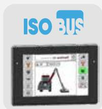
At the first connection the IECU downloads part of the software into the display memory that will be recalled at future vehicle start.
