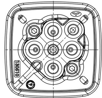
NOTE: normally the pilot control valve is supplied with the handle oriented towards port nr. 4 (see page 20)
