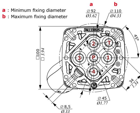
NOTE: normally the pilot control valve is supplied with the handle oriented towards port nr. 4 (see page 28)
