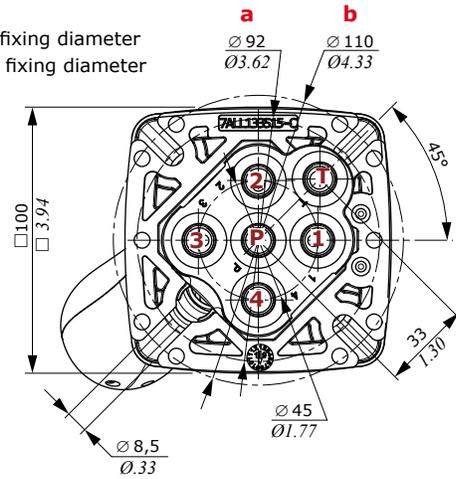
NOTE: normally the pilot control valve is supplied with the handle oriented towards port nr. 4 (see page 28)
