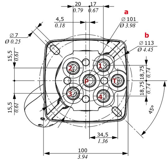
NOTE: normally the pilot control valve is supplied with the handle oriented towards ports nr. 3/4 (see page 28)
