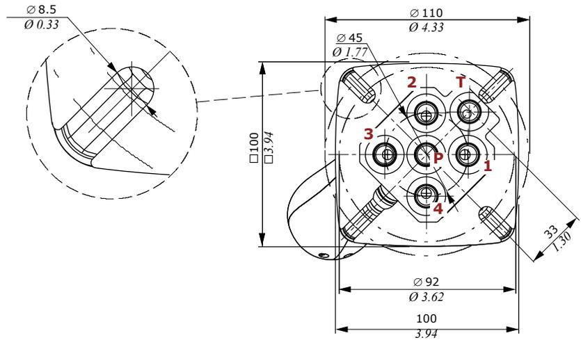
NOTE: normally the pilot control valve is supplied with the handle oriented towards port nr. 4 (see page 28)
