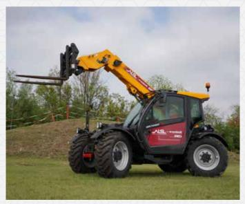
The Agri Farmer 34.7 GD, a more compact and lightweight machine than the Agri Plus used in 2020, is equipped with a single fixed displacement pump and, compared to the previously tested model, benefits even more from the advantages offered by the ALS system.
