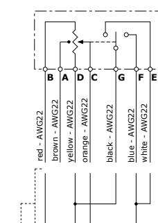
Interface: to use the joystick redundancy option, this wiring is required
