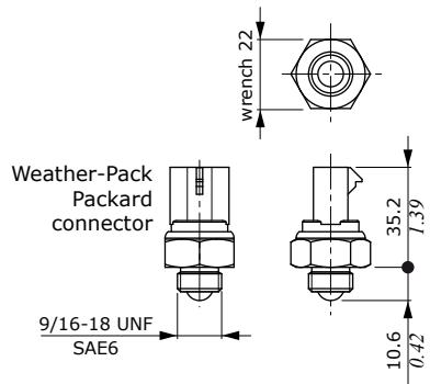
**Sensor with connector and flying leads**
