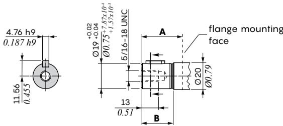
Max transmitted torque = 100 Nm - 74lbft
