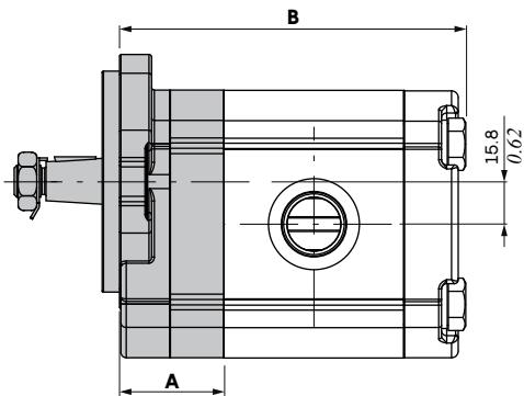
Dimension B is referred to aluminum pump with standard aluminium rear cover (without ports). For SUP flanges dimensions see related pages
