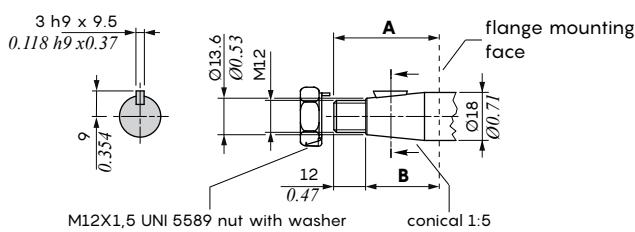
Max transmitted torque = 140 Nm - 103 lbft
