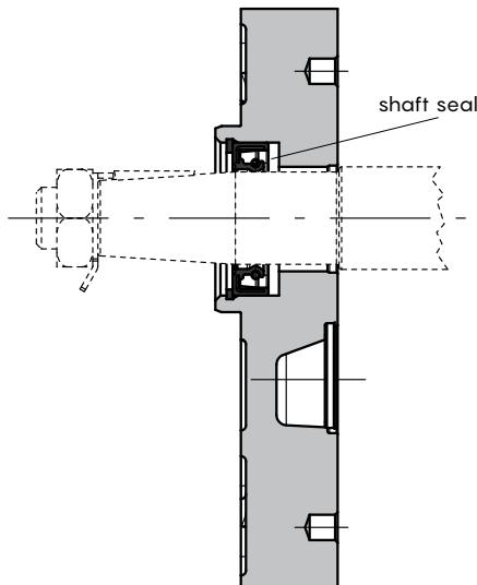
**With shaft seal and dust seal**
