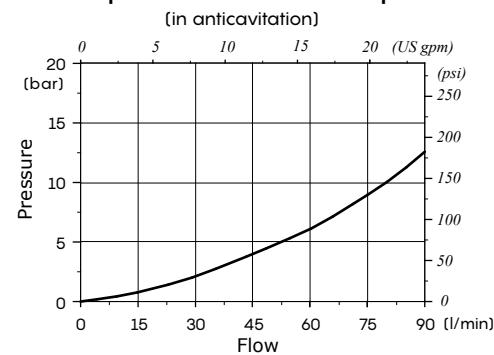
Anti-cavitation valve pressure drop
