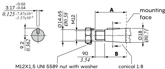
Max transmitted torque = 140 Nm - 103 lbft
