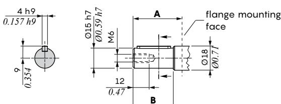
Max transmitted torque = 80 Nm - 59 lbf·ft
