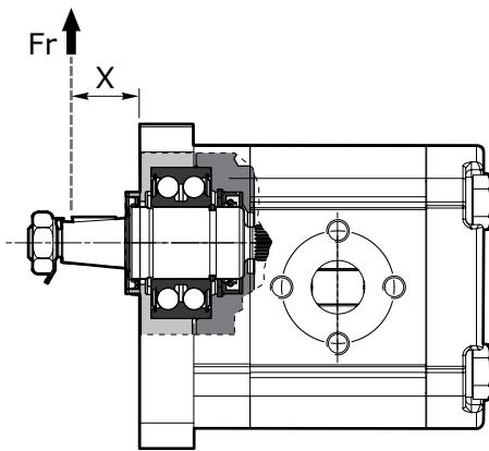
**X** - Distance of the radial load result from the mounting flange mm (in)
