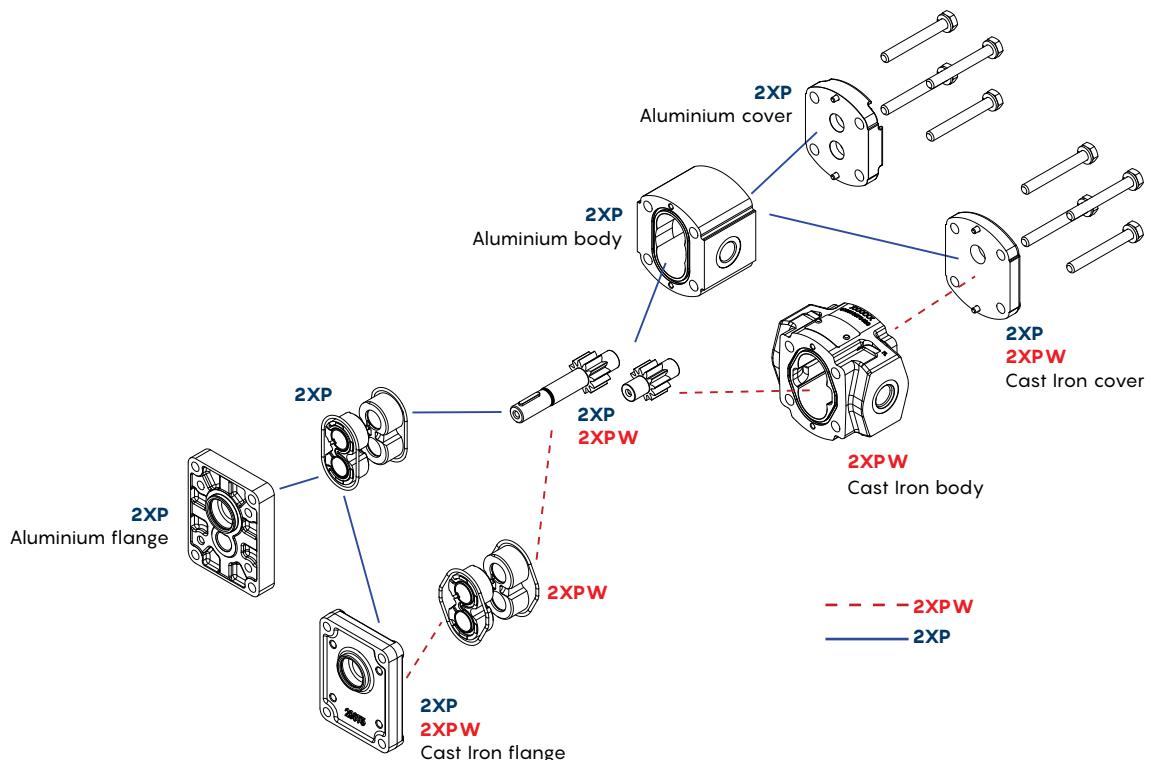
Xtreme is available with aluminium body options (2XP) and cast iron body options (2XPW) and has a complete new set of gear, improving compactness & flexibility. A new generation of plates is able to succeed in the most demanding applications.
