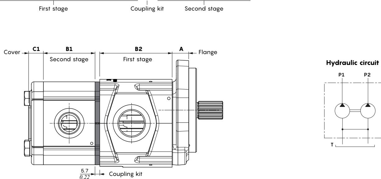
**2XP or 2XPW primary stage****2XP/2XPW - TK tandem dimensions****2XPW double stage description example****2XPW-G-190-D-EUR-B-N-10-0-G34G12/TK /2XPW-G-190-0-G34G12**
