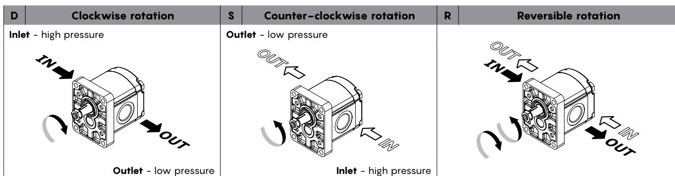
**Pump/motor rotation reversal****How to invert the wise rotation:**
