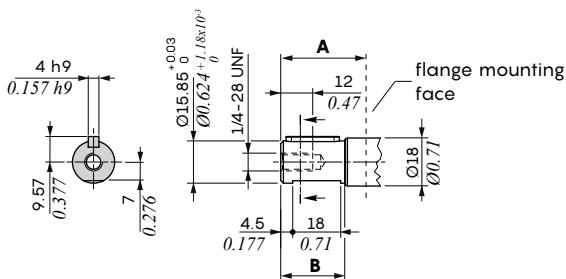
Max transmitted torque = 90 Nm - 66 lbf·ft
