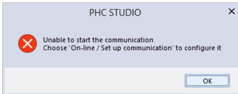
Missing of the RS232 adapter or driver or wrong COM port setted.
